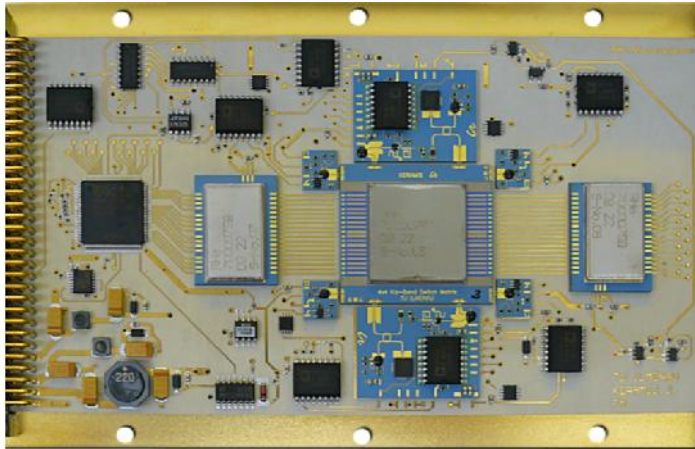
Digitally controllable switch-matrix circuit board
