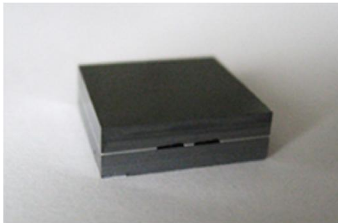
Oil cuvette made of silicon and LTCC
