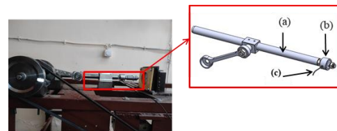
Fig. 2. The combination of the sensor and the test bench (a): travel shaft, (b): force sensor, (c): 4-conductor connecting cable
