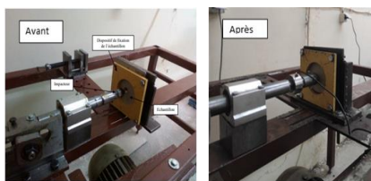
Fig. 5. Sample fixing system before and after modification
