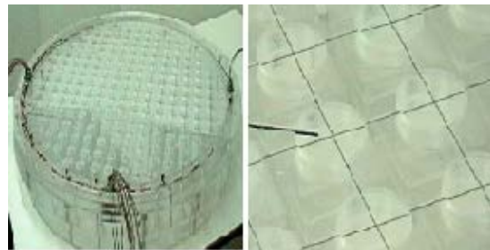
Fig 6 Wire mesh sensor at the core entrance
