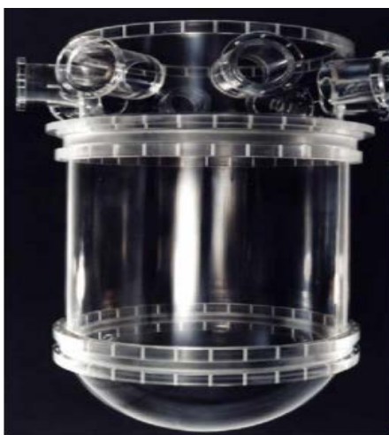
Fig.1 Perspex model of the RPV in ROCOM
