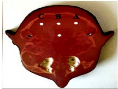
Fig 3 Phantom slice on which the dosimeters are placed Top: Bottom face
