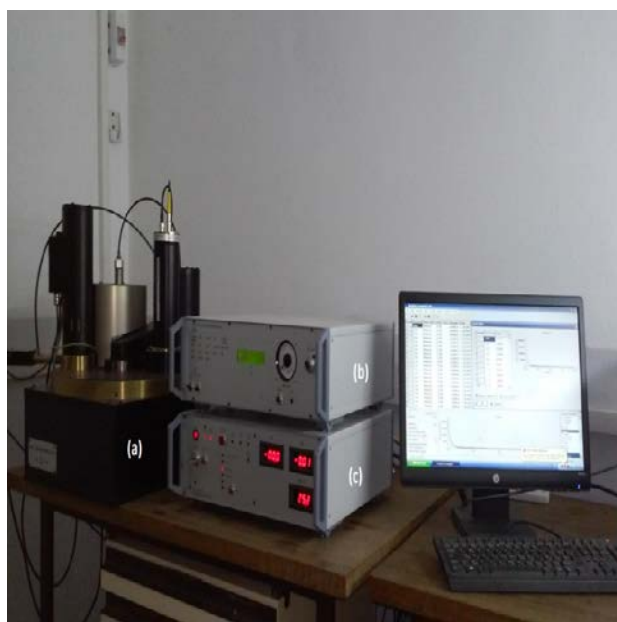
Fig. 1 Used RISØ TL/OSL-DA20 Reader, a) Reader, b) Controller, c) The X-ray generator controller
