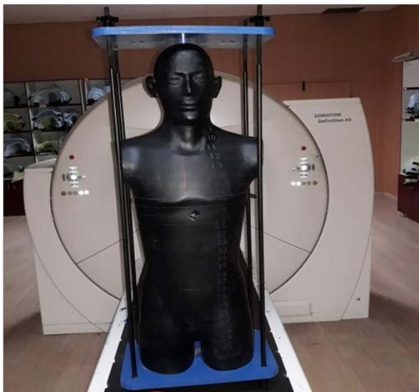
Fig. 1 Used male ART representing a man 175 cm high and 73.5 kg in weight
