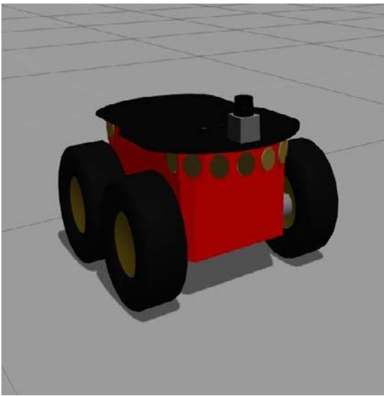
Fig.5 Gazebo Model of P3-AT with LRF Attached
