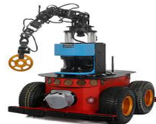
Fig.1 Pioneer P3-AT equipped with arm manipulator
