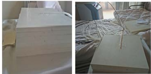
Fig.3 Applicator and Gafchromic film disposition on phantom
