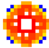
Fig.2 Fission source spatial distribution for the reactor mid-plane (z=0)
