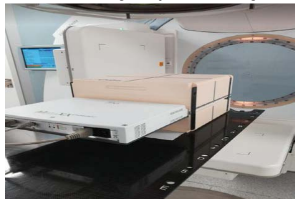
Fig. 3: MatriXX Evolution associated with multicub phantom (Oncopole clinic)
